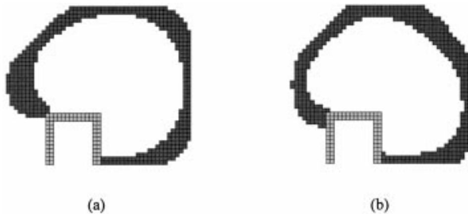
Fig. 13. Optimized cross sections (25% mass constraint): (a) w_J = 1.0 and w_I = 0.0 ; (b) w_J = 1.0 and w_I = 0.4 .
