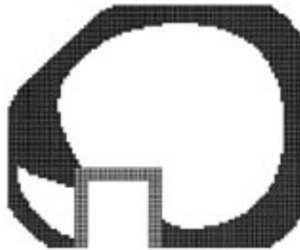
Fig. 12. Optimized cross section with the half size of the original mesh used for Fig. 10(a).
