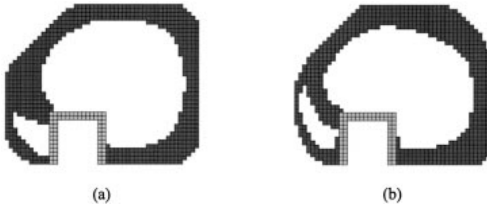
Fig. 10. Optimized cross sections (40% mass constraint): (a) w_J=1.0 and w_I=0.0 ; (b) w_J=1.0 and w_I=0.4 .
